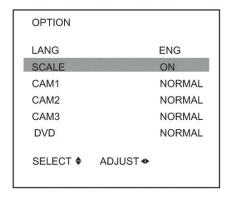
Press  $\triangle \odot / \nabla \odot$  to select ON / OFF. Scale refers to the reversing distance indicator displayed on the monitor.
