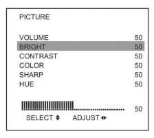
Press  $\triangle$  O / $\nabla$  O to adjust the BRIGHTNESS level.
