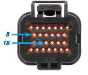
Insert the orange and yellow wires into Socket 8 & 16.
