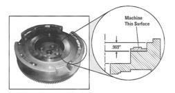
If flywheel step is .787 (20mm) but is a stepped surface, the flywheel step must be machined to .969 (24.6mm) use PTO disc A-RE72536SPL
