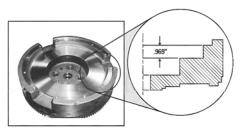
If the flywheel step is .969 (24.6mm) use PTO disc A-RE72536SPL
