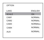
Press  $\Delta \odot / \nabla \odot$  to select ON/OFF. Scale refers to the reversing distance indicator displayed on the monitor.
